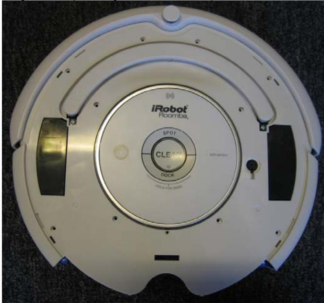
**Top View (top chassis +user panel removed)**
