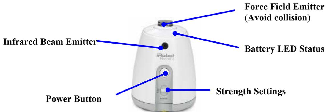
The Virtual Wall beam is triangular shaped. A small halo prevents Roomba from bumping into the Virtual Wall and a larger cone-shaped section blocks off areas of your home where you don't want Roomba to go.
